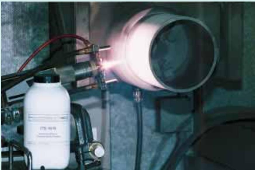
**Figure 67** Thermal spraying of a Ceramer/Silicon Aluminum mixture.
