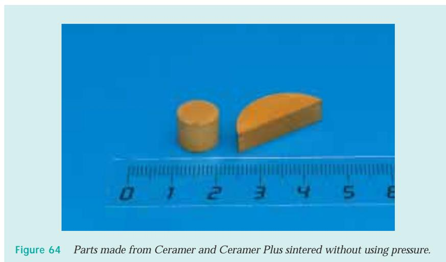
Figure 64 Parts made from Ceramer and Ceramer Plus sintered without using pressure.
